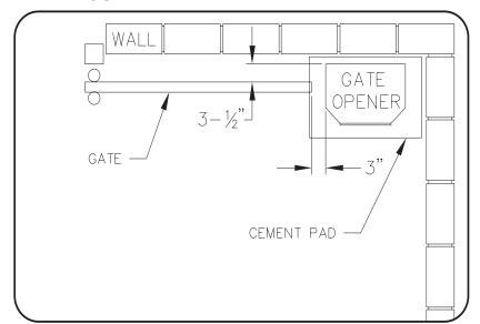
O The rear mount installation is an excellent way to conceal the chain or operator. The operator is placed in the extreme rear of the gate as shown and the chain never goes across the driveway. The chain only goes from the gate operator to a post or wall beside the driveway. Place shortest edge of the operator 3" from the rear end of the gate and place the long edge of the operator 3-1/2" away from the gate toward the wall.
